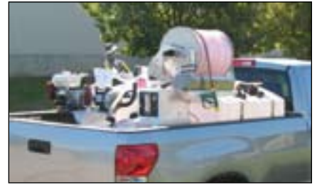
Spray rig on open deck truck fitted with CF Valves
