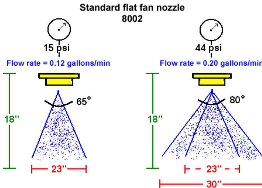
Figure 2A: Pressure fluctuations and its effect on spray angle.
