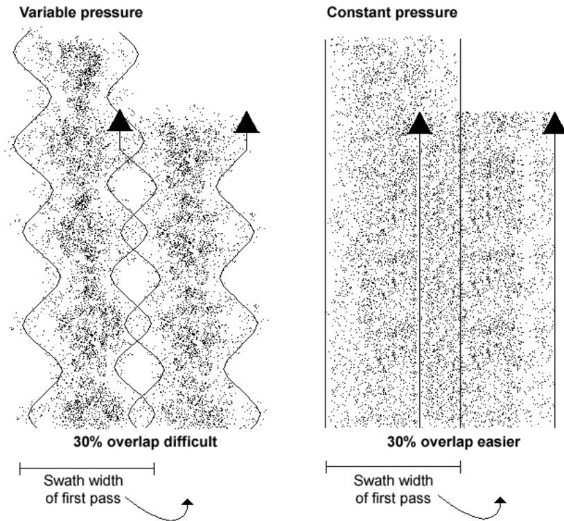
Figure 2B: Pressure fluctuations and its effect on swath width.
