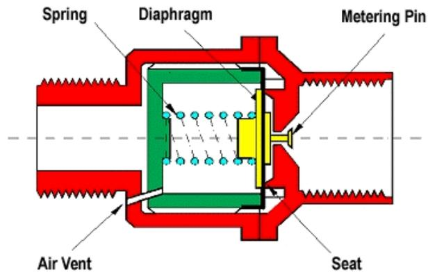
Figure 4. Cross-section of CFValve™ (with permission of Sprays International Ltd.)
