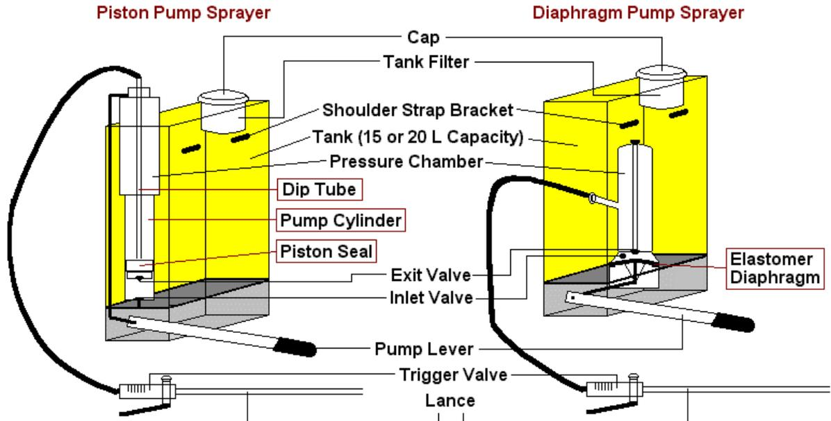
Figure 1. Structural components of a knapsack sprayer.
