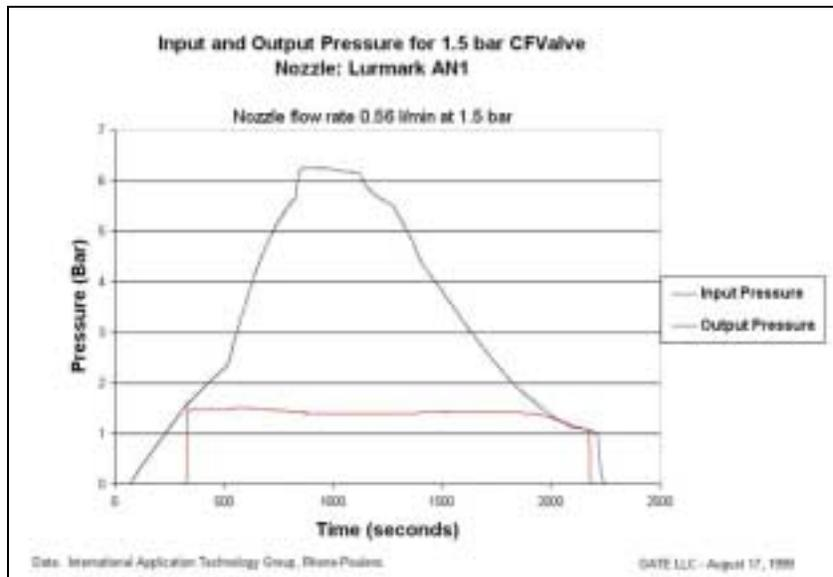
Figure 5. Input and output pressure for a 1.5 bar CFValve™ with a Lurmark AN1 nozzle.
