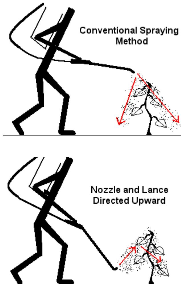
Figure 6. Conventional and upward pointed nozzle spraying methods.
